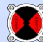
ACTUADOR CERRADO ACTUATOR CLOSED
