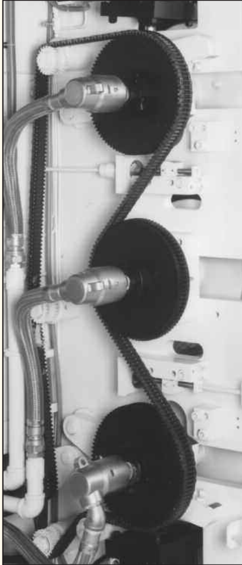
Main drive on plastic film extruder
